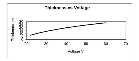
Thickness variation can be controlled within 20% at 10 $\mu$ m, to 10% at 20 $\mu$ m with appropriate control of the system.
